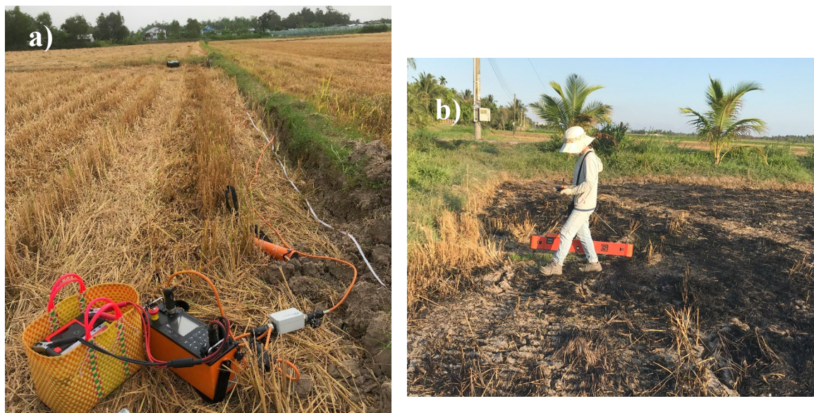
Figure 2 Soil salinity measurement in situ using geo-physics methods: a) ARES II, b) EM38-MK2.
