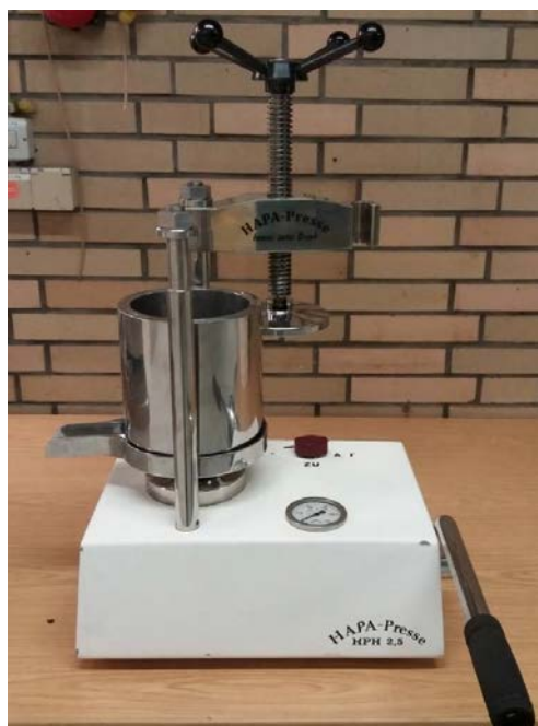
Figure 2. A hydraulic tincture press used for the digestate separation experiments in the laboratory.
