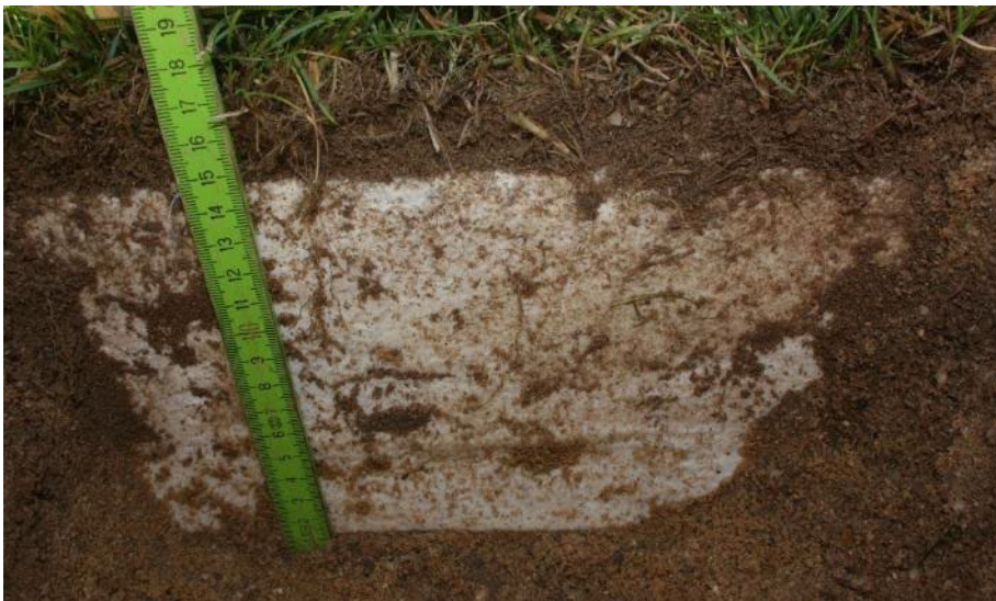
Figure 3-3: Incorporated nonwoven connecting rootzone layer and drainage layer in one of the test plots. (© B. Stürmer-Stephan)
