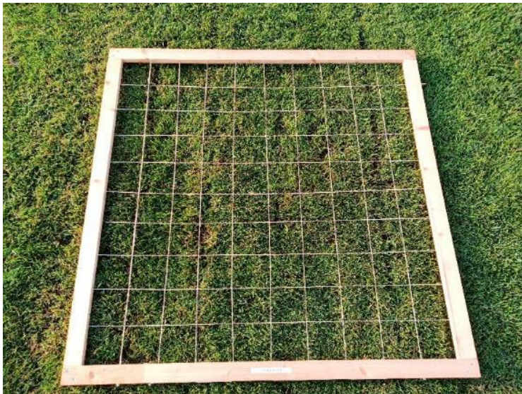
Figure 3-6: Wooden frame according to DIN 12231 (2003) on a part of the treated turf. The closed slits can be recognized. (© B. Stürmer-Stephan)
