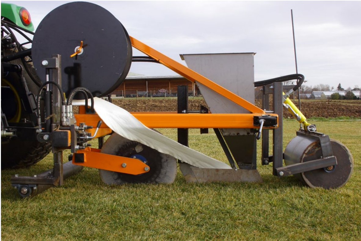
Figure 3-5: The developed device incorporates a 150 mm height nonwoven in a depth of 170 mm on one of the test plots. The box above the coulter can be used for testing the incorporation of additional sand, but this feature is not investigated within this work. (© B. Stürmer-Stephan)
