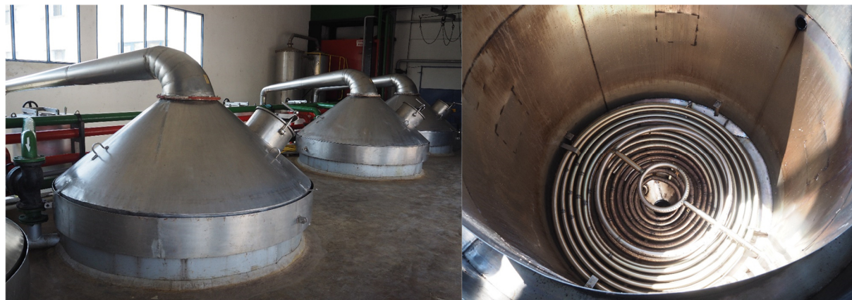
Figure 1. Representative distillation apparatus as used to produce various essential oils. Here for rose essential oil production in Bulgaria. © Sonja Schrack-Belschner.
