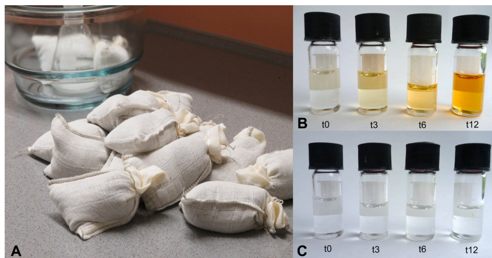
Fig. 2. Caraway seeds in sewed linen bags (14 × 8 cm) stored in a desiccator (A). Carvone stored for 0, 3, 6 and 12 months at 40 °C in the dark (B). Limonene stored for 0, 3, 6 and 12 months at 40 °C in the dark (C).
