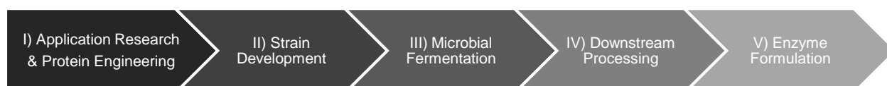
Figure 10: Flowchart of the five general stages of microbial enzyme production (adapted from Dodge) [32].
