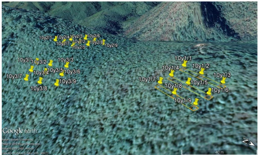
Figure 4: Example of plot lay-out and soil sampling points of 10-year fallow in Nong Khao. Field codes: 10y = 10-year fallow age. Second number = hill ID. Last number = sampling point ID of each hill. Yellow rectangular plots for tree community survey size were 6 x 50 m. Orange rectangular plots for surveys of indicator trees of soil properties size were 5 x 6 m. Source: Google Earth Pro. Image Date: 12/11/2015.
