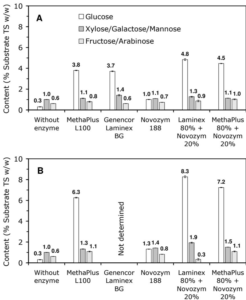
**Figure A3.** Concentration of soluble monosaccharides after enzymatic hydrolysis of ensiled maize straw in the screening experiment [Hydrolysis of 1.8 g maize straw in 10 mL of water at pH 3.6 and 55°C for 24 hours. n=2. Vertical arrows stand for SD. (A) 13 g/kg substrate VS; (B) 130 g/kg substrate VS].
