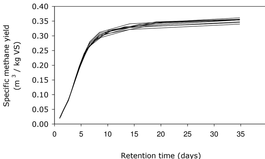
**Figure 28.** Methane production of ensiled maize straw [Digestion temperature: 37°C. Average values. n=3].
