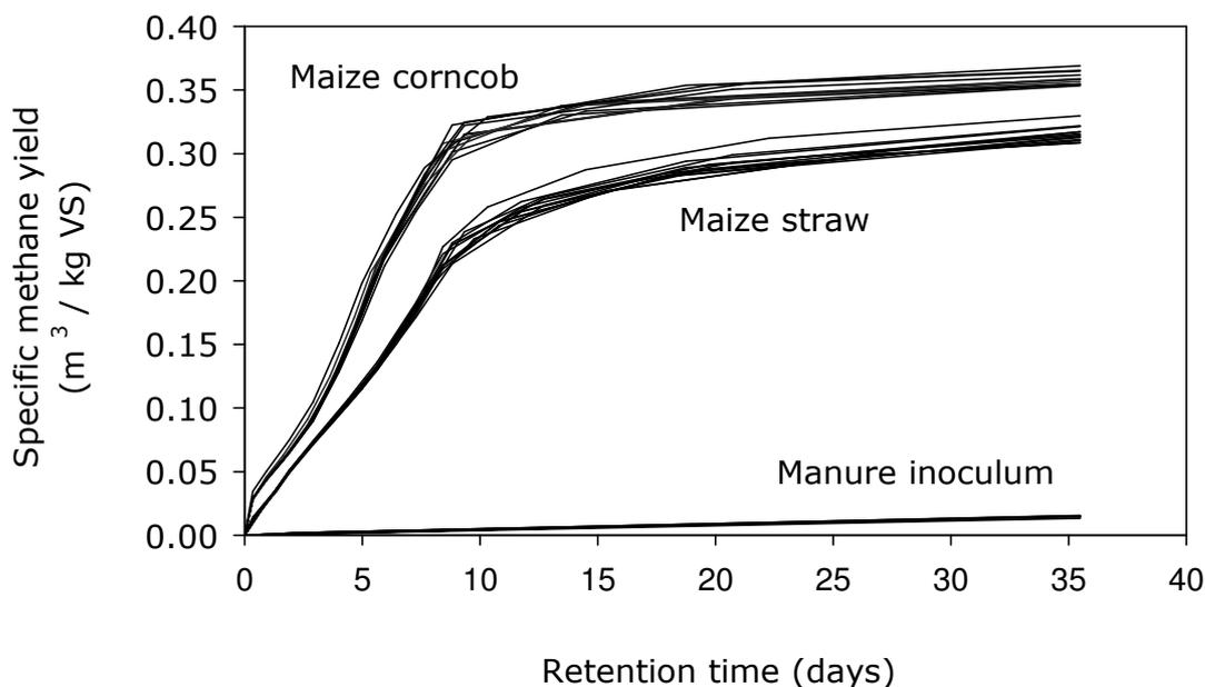
**Figure 22.** Methane production of corncob, maize straw, and manure inoculum [All variants with and without enzyme addition. Average values. n=3. Digestion temperature 37°C. Numerical values cf. Appendix A 4].
