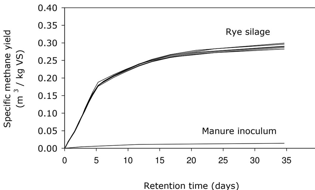
**Figure 23.** Methane production of coarse rye silage and manure inoculum [All variants with and without enzyme addition. Average values.  $n \geq 2$ . Digestion temperature 37°C. Numerical values cf. Appendix A 4].
