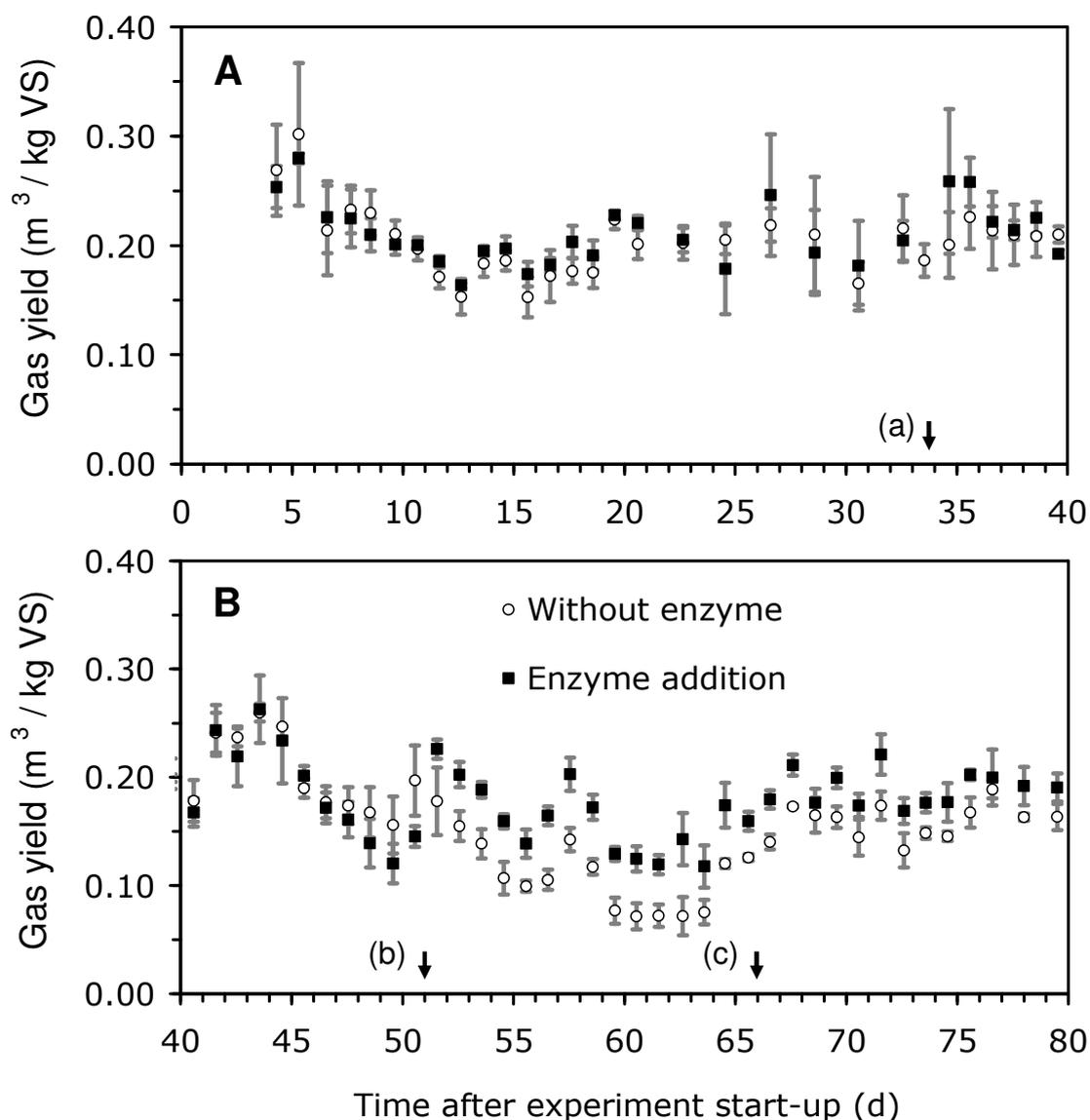
**Figure 33.** Specific gas yield during acidogenic fermentation with and without enzyme addition [Average values. n=4. Vertical arrows stand for SD. (a) HRT reduced from 10 to 5 days. (b) Enzyme additive MethaPlus L100 10 g/kg VS. (c) Enzyme additive 1 g/kg VS].
