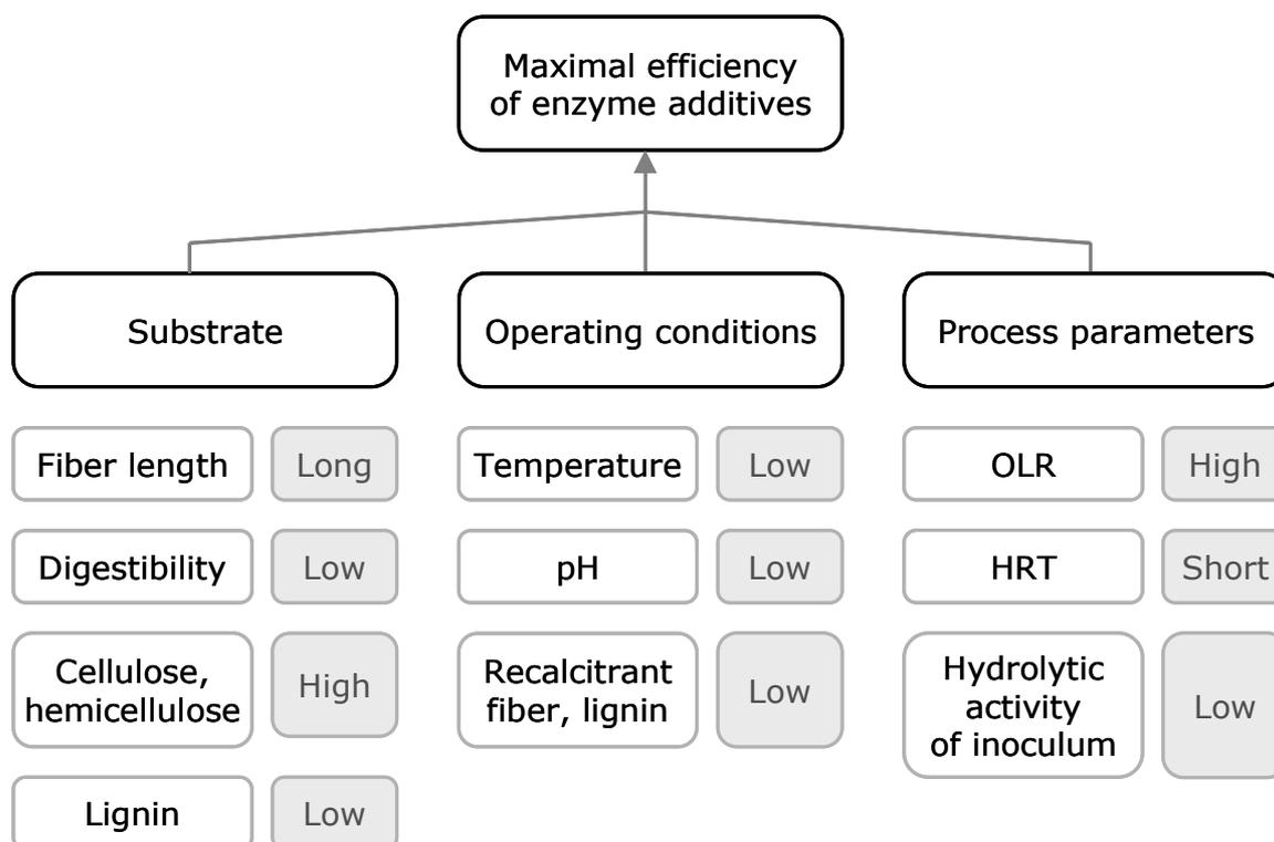
**Figure 36.** Requirements for maximal efficiency of enzyme additives in anaerobic digestion processes.
