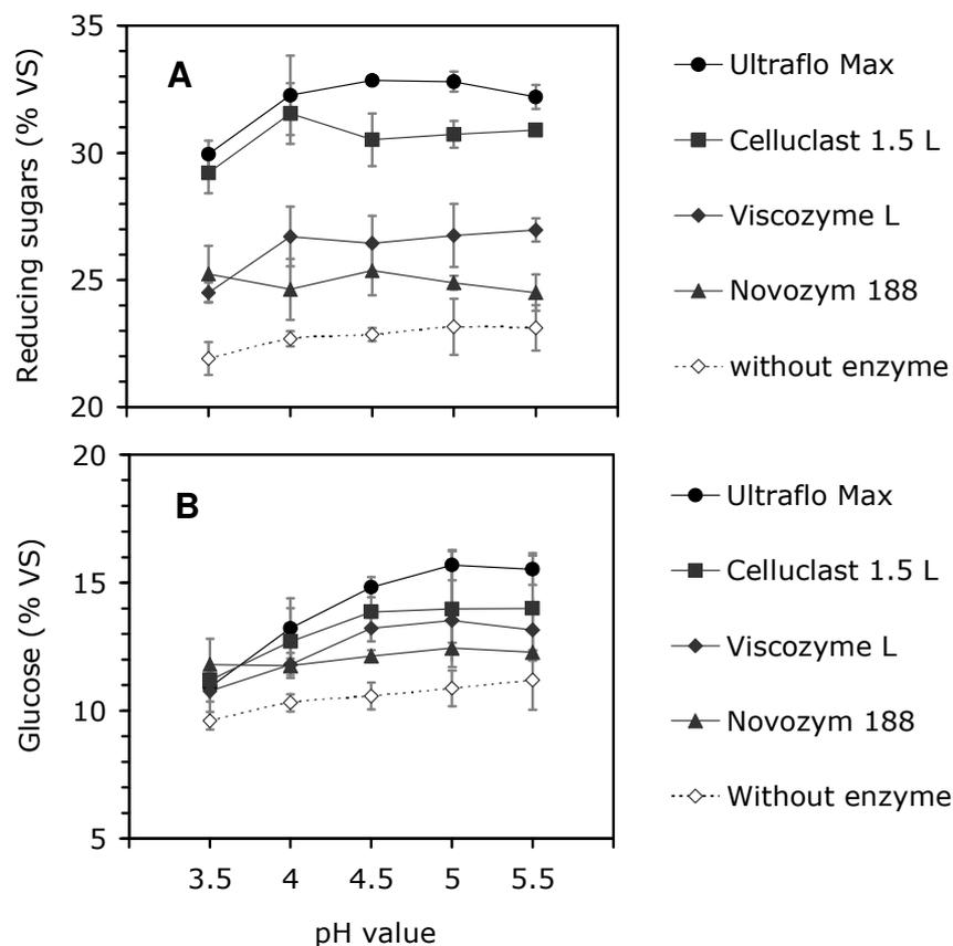
**Figure A2.** Reducing sugars (A) and glucose (B) release from maize straw at different pH values [Hydrolysis of 1.8 g maize straw with 10  $\mu$ L enzyme solution in 10 mL of 0.1 M citrate buffer solution at 50°C for 24 hours. n=3. Vertical arrows stand for SD. Numerical values of glucose assay cf. **Table A8**].
