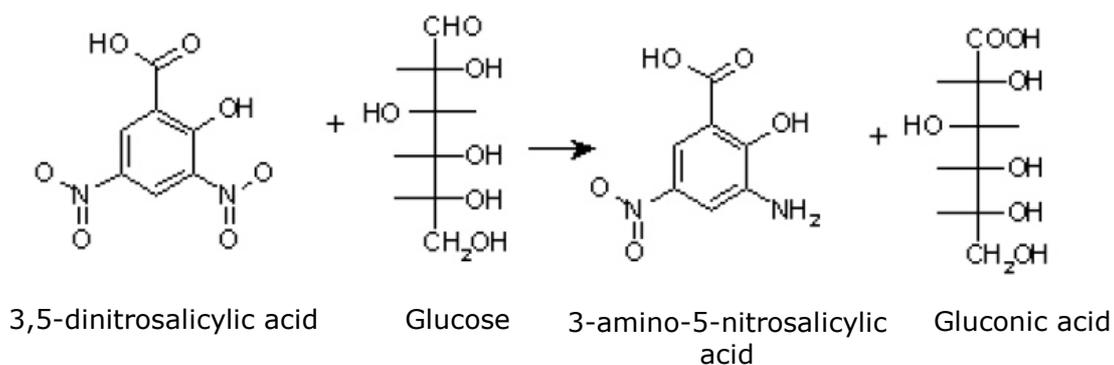
**Figure 2.** Reaction of glucose with dinitrosalicylic acid.
