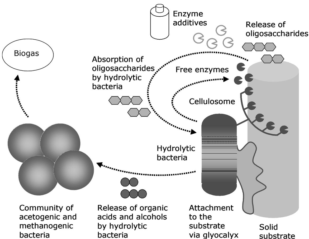
**Figure 35.** Mechanisms of lignocellulosic substrate degradation in the biogas process.
