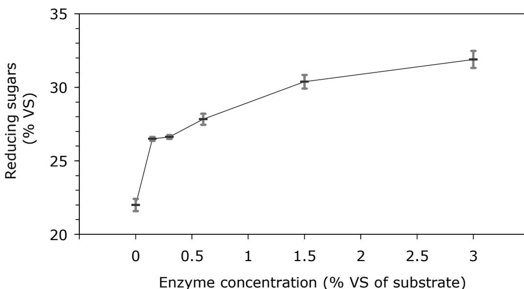
**Figure 20.** Reducing sugars release from maize straw at different enzyme concentrations [Hydrolysis of 1.8 g maize straw in 10 mL of 0.1 M citrate buffer solution for 24 hours at pH 4.5 and 50°C. n=3. Vertical arrows stand for SD. Numerical values cf. Appendix A I].
