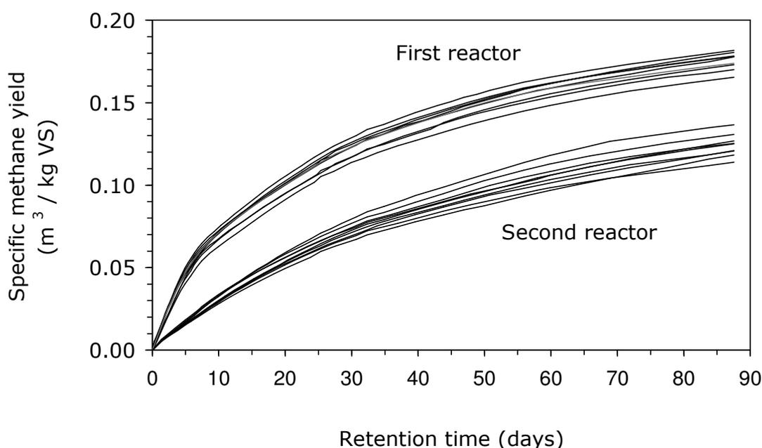
**Figure 29.** Methane production of reactor samples digested at 37°C [Average values. n=3. Enzyme products: MethaPlus L100 or Novozym 342/Pulpzyme HC (50/50 w/w). Enzyme dosages: 0.2 (low) or 2 g/kg FW (high). Dosage divided into 20 additions performed every ~3 days from the start of the digestion period].
