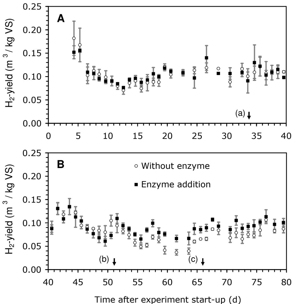
**Figure 34.** Specific biohydrogen yield of gas during acidogenic fermentation with and without enzyme addition [n=4. Vertical arrows stand for SD. (a) HRT reduced from 10 to 5 days. (b) Enzyme additive MethaPlus L100 10 g/kg VS. (c) Enzyme additive 1 g/kg VS].
