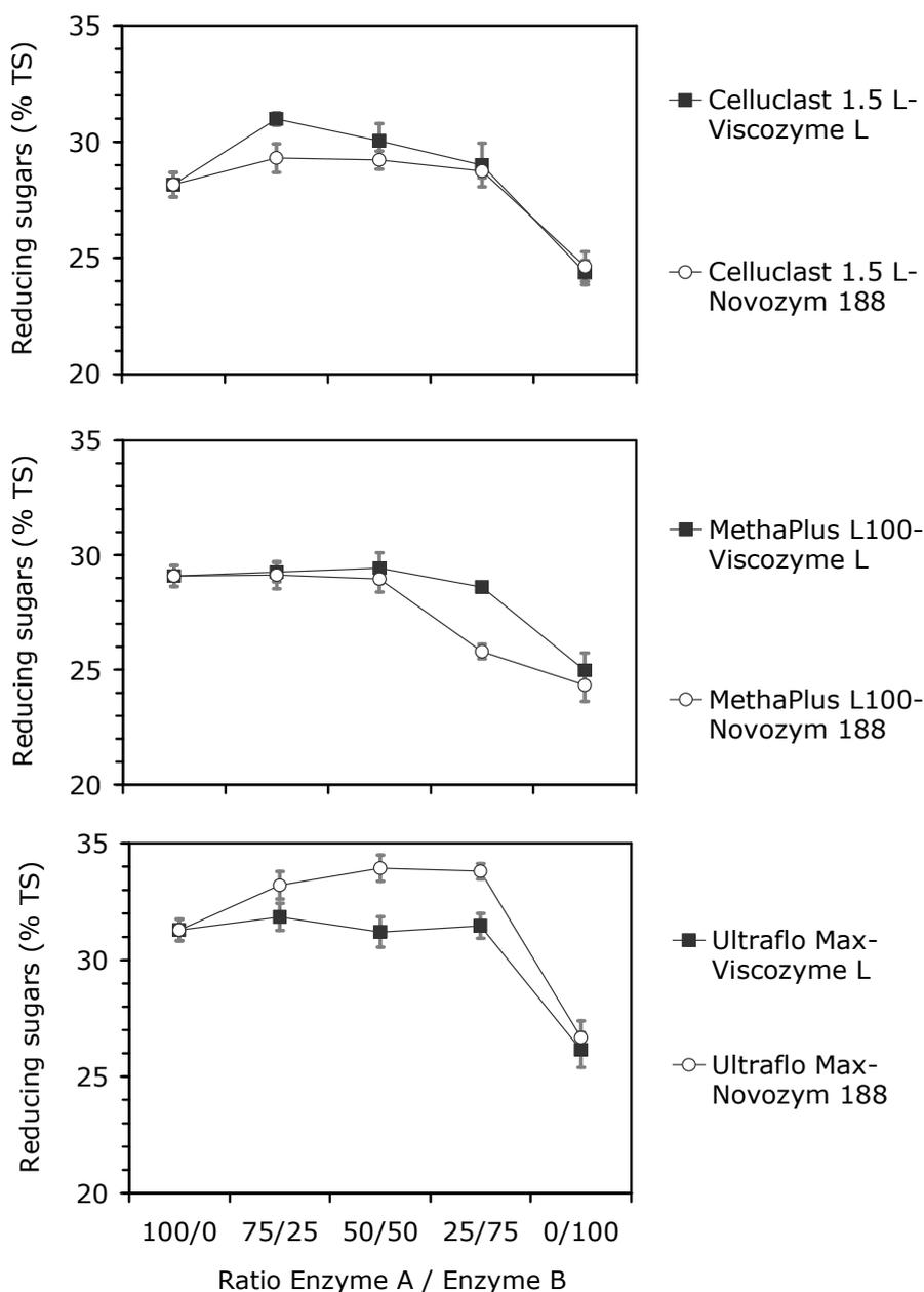
**Figure 18.** Reducing sugars release from maize straw with different enzyme mixtures [Hydrolysis of 1.8 g maize straw with 10  $\mu$ L enzyme mixture in 10 mL of 0.1 M citrate buffer solution for 24 hours at pH 4.5 and 50°C. n=3. Vertical arrows stand for SD. Numerical values cf. Appendix A I].
