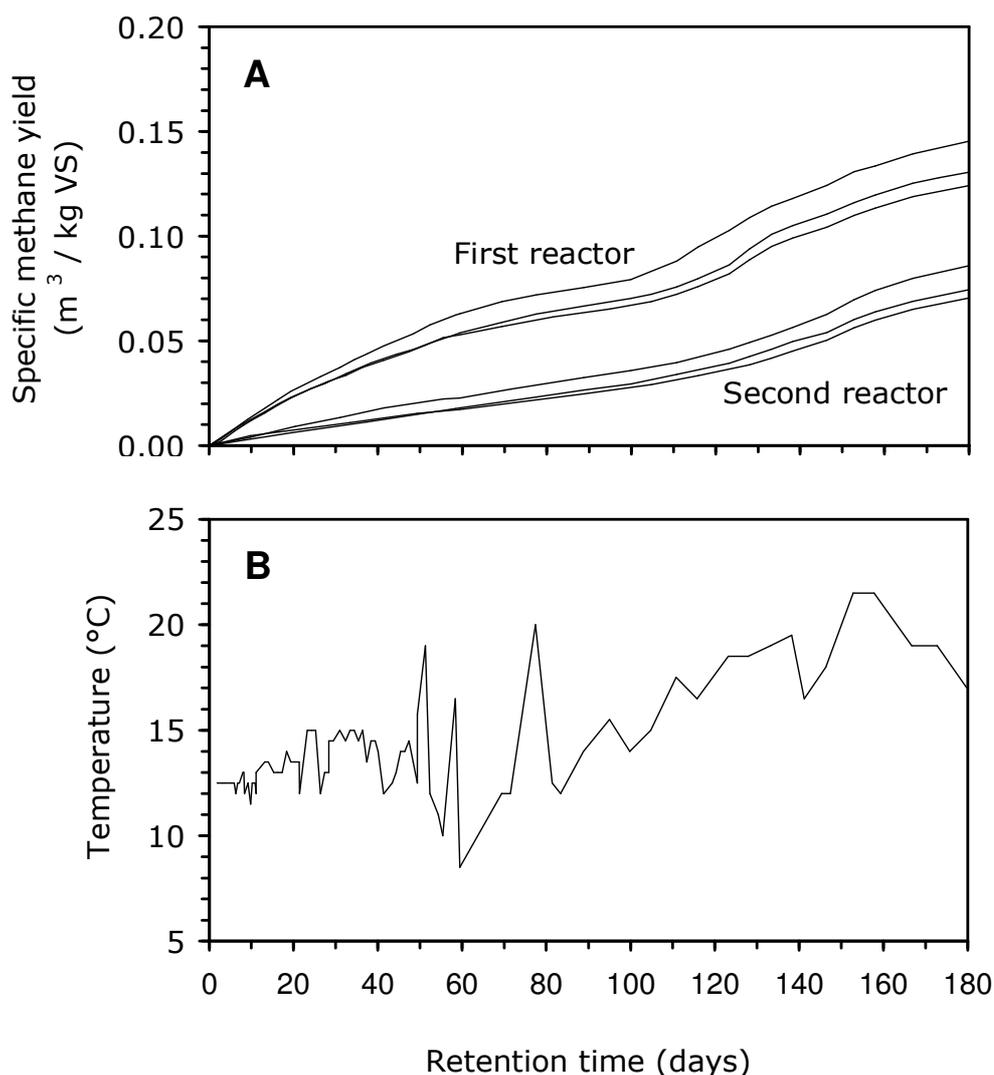
**Figure 30.** Methane production (A) and temperatures (B) of reactor samples digested at room temperature [Average values. n=3. Enzyme products: MethaPlus L100 or Novozym 342/Pulpzyme HC (50/50 w/w). Enzyme dosage: 2 g/kg FW. Dosage divided into 20 additions performed every ~3 days from the start of the digestion period].
