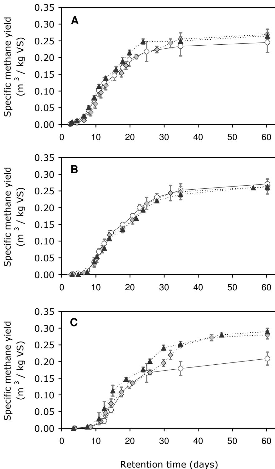
**Figure 26.** Methane production of coarse grass silage incubated with diluted inoculum [Average values. n=2. Vertical arrows stand for SD. Standard inoculum diluted 3-fold (A), 5-fold (B) and 10-fold (C). Addition of enzyme product MethaPlus L100 at low (0.7 g/kg VS) and high enzyme dosage (7 g/kg VS). Numerical values cf. Appendix A 4].
