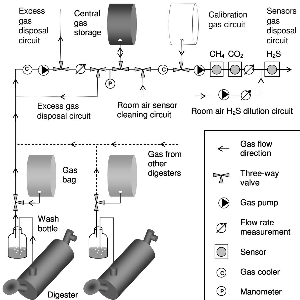
**Figure 8.** Automatic gas measurement system for continuous experiments.
