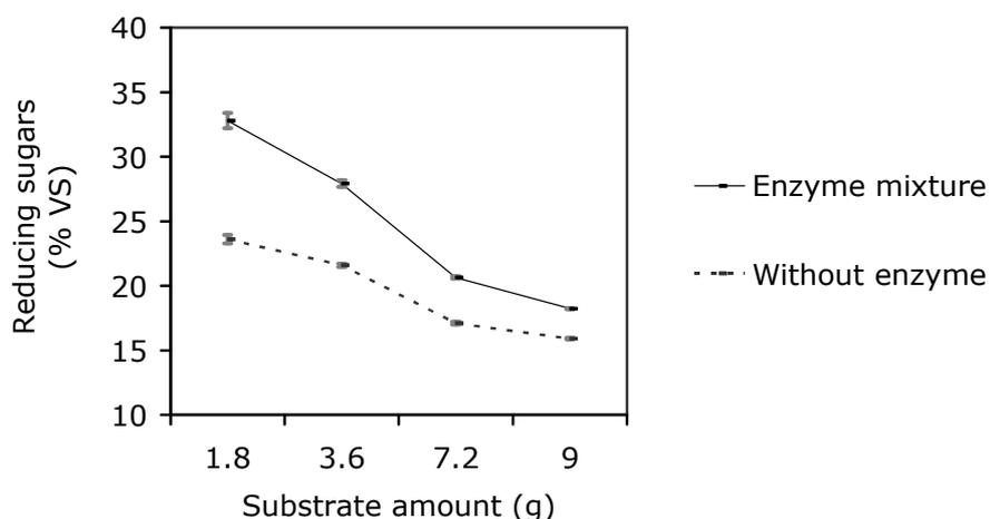
**Figure 21.** Reducing sugars release from maize straw at different substrate concentrations [Hydrolysis of maize straw with 10  $\mu$ L enzyme mixture in 10 mL of 0.1 M citrate buffer solution for 24 hours at pH 4.5 and 50°C. n=3. Vertical arrows stand for SD. Numerical values cf. Appendix A I].
