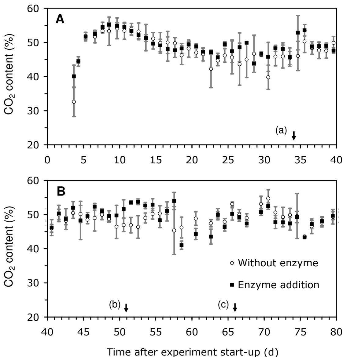
**Figure 32.** Carbon dioxide content of gas during acidogenic fermentation [Average values, n=4. Vertical arrows stand for SD. (a) HRT reduced from 10 to 5 days. (b) Enzyme additive MethaPlus L100 10 g/kg VS. (c) Enzyme additive 1 g/kg VS].
