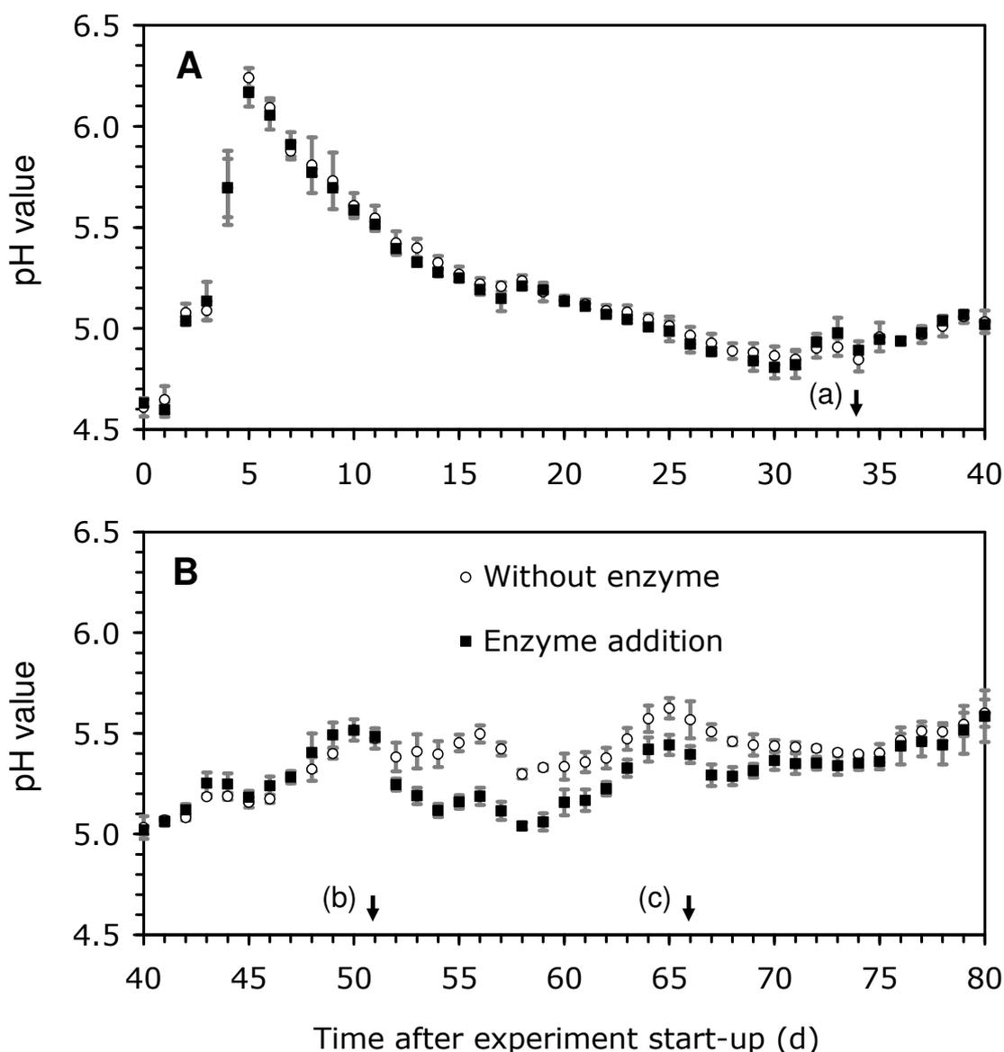
**Figure 31.** pH of digesters during acidogenic fermentation with and without enzyme addition [Average values.  $n=4$ . Vertical arrows stand for SD. (a) HRT reduced from 10 to 5 days. (b) Enzyme additive MethaPlus L100 10 g/kg VS. (c) Enzyme additive 1 g/kg VS].
