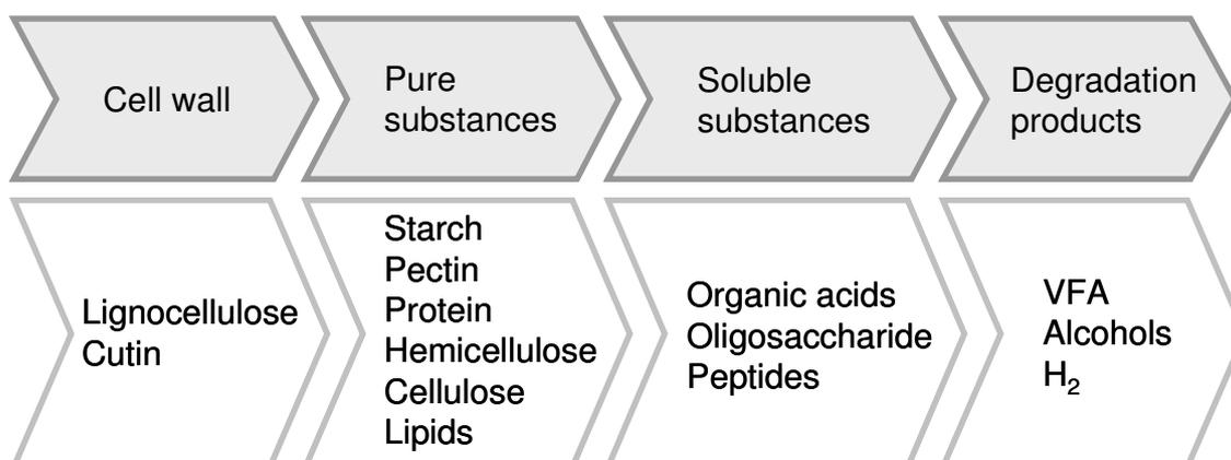
**Figure 1.** Classification of molecules in increasing order of degradability [Compiled after Hobson and Wheatley (1993), Tong et al. (1990), Jung and Engels (2002)].
