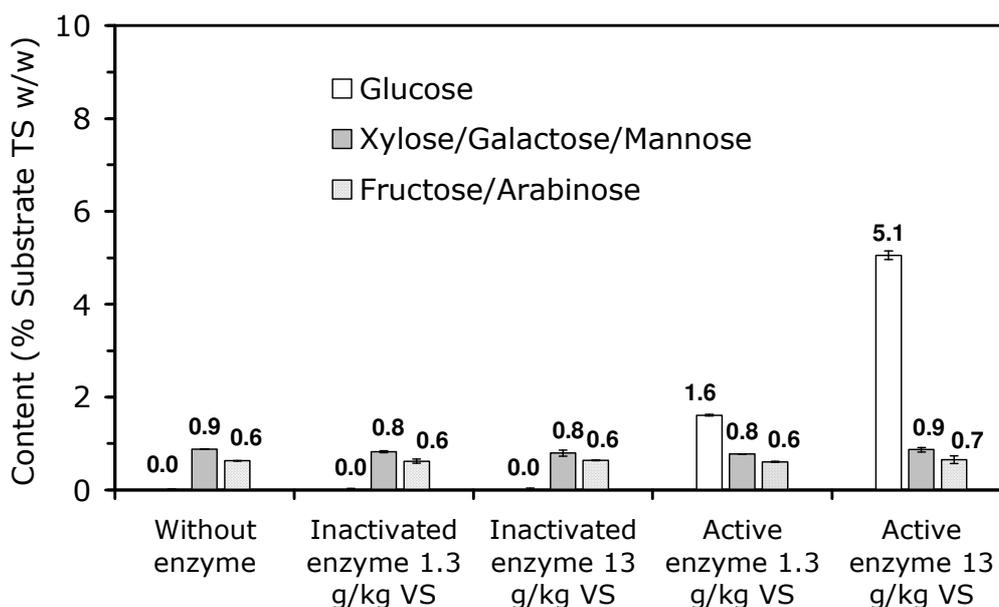
**Figure 27.** Concentration of soluble monosaccharides after enzymatic hydrolysis of ensiled maize straw as a pretreatment step before anaerobic digestion [Hydrolysis of 1.8 g ensiled maize straw in 10 mL of water at pH 4.5 and 45°C for 24 hours. Application of enzyme mixture Genencor Laminex BG / Novozym 188, respectively 80% and 20% (w/w). n=2. Vertical arrows stand for SD].
