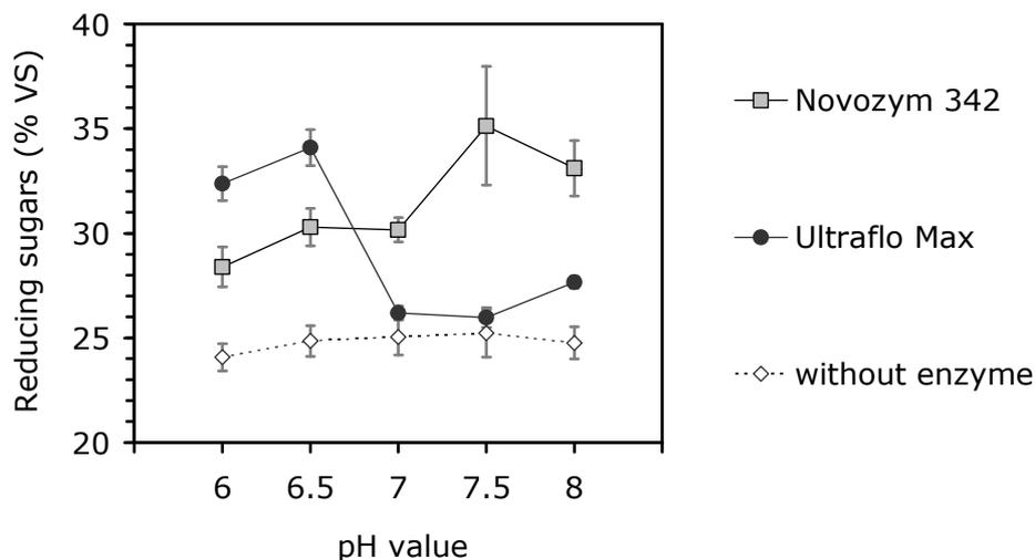
**Figure 16.** Reducing sugars release from maize straw at neutral pH values [Hydrolysis of 1.8 g maize straw with 10  $\mu$ L enzyme solution in 10 mL of 0.1 M citrate buffer (pH 6) and phosphate buffer (pH 6.5-8) solution at 50°C for 24 hours. Addition of sodium azide at 1 g/L in each sample for bacterial inhibition. n=3. Vertical arrows stand for SD. Numerical values cf. Appendix A I].
