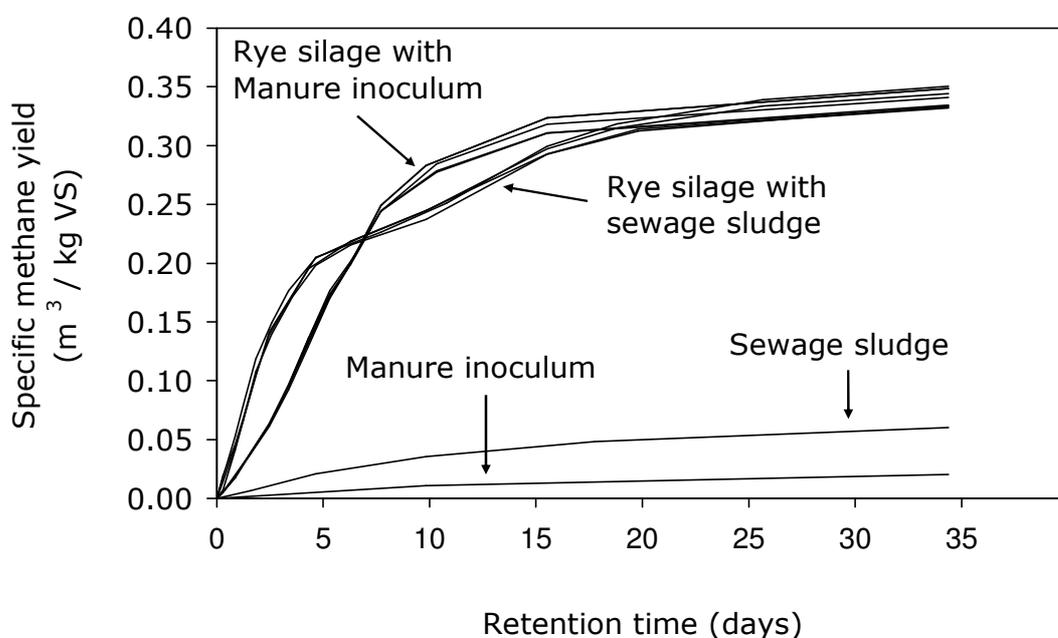
**Figure 24.** Methane production of finely ground rye silage and manure inoculum [All variants with and without enzyme addition. Average values.  $n=3$ . Digestion temperature  $37^{\circ}\text{C}$ ].
