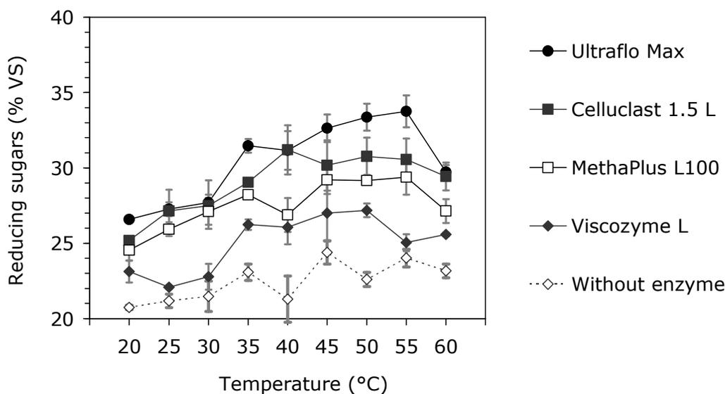
**Figure 17.** Reducing sugars release from maize straw at different temperatures [Hydrolysis of 1.8 g maize straw with 10  $\mu$ L enzyme solution in 10 mL of 0.1 M citrate buffer solution at pH 4.5 for 24 hours. n=3. Vertical arrows stand for SD. Numerical values cf. Appendix A I].
