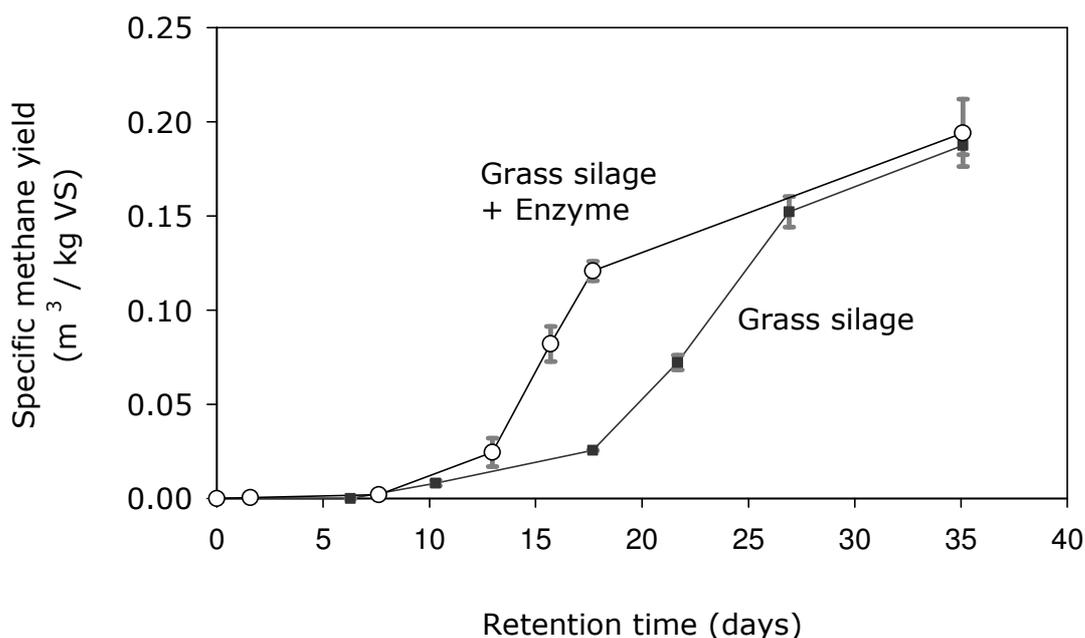
**Figure 25.** Methane production of coarse grass silage incubated with weak inoculum [Average values. n=2. Vertical arrows stand for SD. Enzyme dosage of MethaPlus L 100 in variant with enzyme addition: 11 g/kg VS. Digestion temperature 37°C. Numerical values cf. Appendix A 4].
