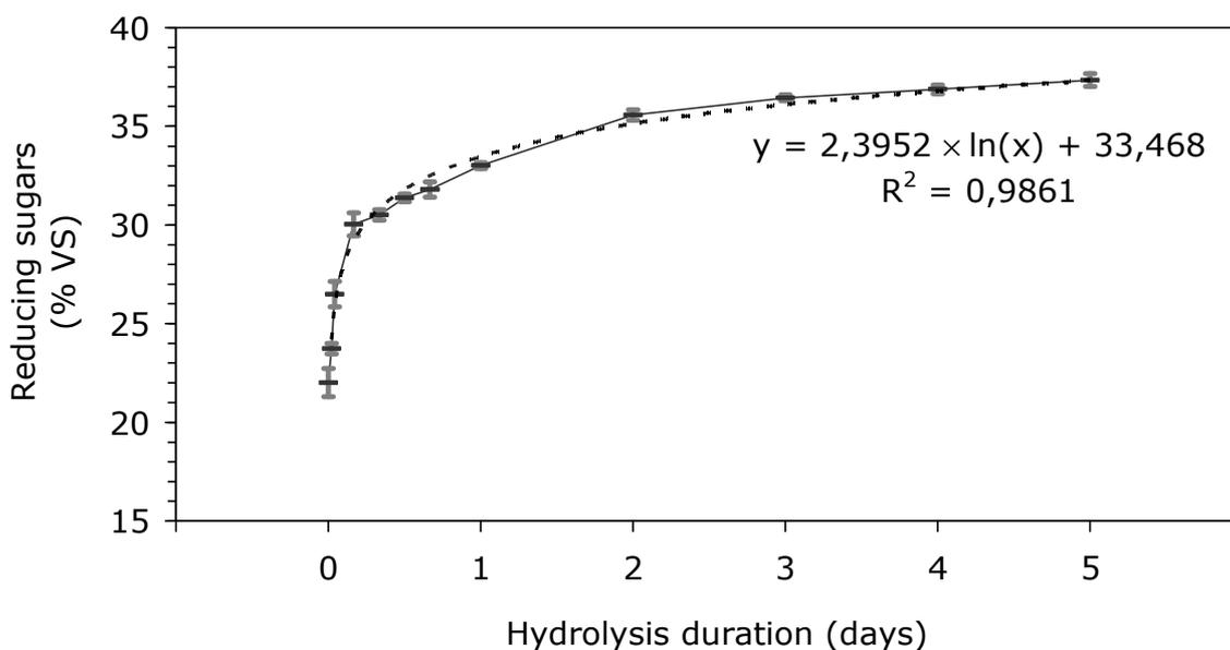
**Figure 19.** Reducing sugars release from maize straw at different durations [Hydrolysis of 1.8 g maize straw with 10  $\mu$ L enzyme solution in 10 mL of 0.1 M citrate buffer solution for 24 hours at pH 4.5 and 50°C. n=3. Vertical arrows stand for SD. Numerical values cf. Appendix A I].
