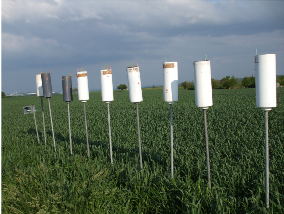
Fig 2: Exposure of bioindicator plants and passive diffusion tube samplers at a site in the field.
