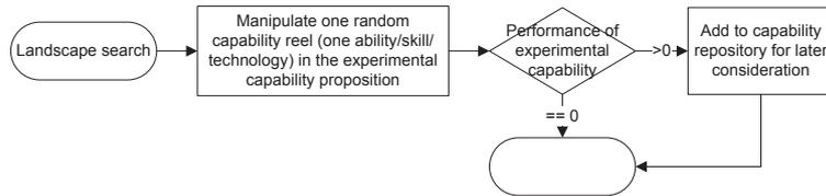
Figure 4: Flowchart of operational landscape search in which the experimental capability is manipulated to find new feasible capabilities by trial-and-error.
