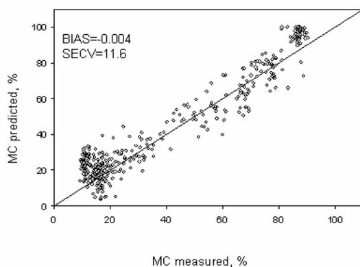
Fig. 5. Prediction models for moisture content (MC) based on backscattering area
