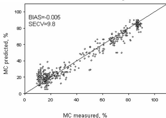
Fig. 6. Prediction models for moisture content (MC) based on Light luminescence
