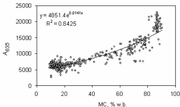
Fig. 3. Relationship between moisture content (MC) with backscattering area (A635)
