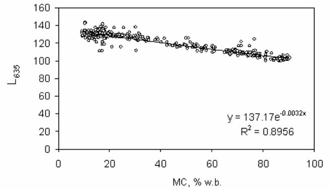
Fig. 4. Relationship between moisture content (MC) with backscattering area (A635)
