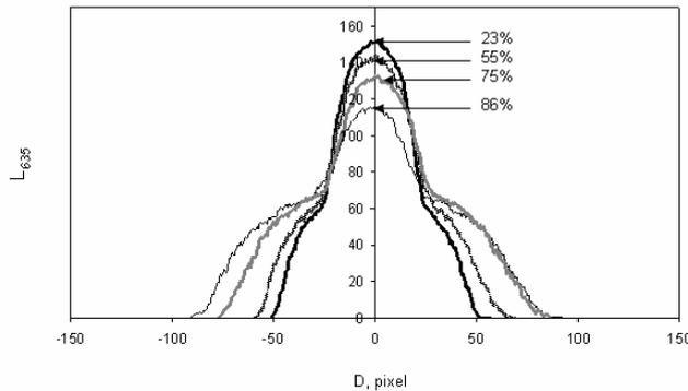
Fig. 2. Light luminescence at 635 nm (L635) versus scattering diameter (D) in apple tissue at different moisture content.
