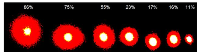
Fig. 1. Laser scattering images at 635 nm wavelength at different levels of moisture content (MC, % w.b.).
