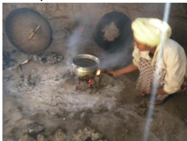
Fig. 7. WBT with dung cake as fuel
