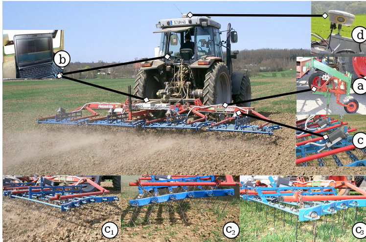
Figure 2.3: Prototype of the automatically controlled flexible-tine harrow, modified after Rueda-Ayala et al. (2010). (a) Soil sensor; (b) computing unit; (c) motor; (c 1 ) light intensity; (c 2 ) strong intensity; (c 3 ) strongest intensity; (d) RTK-DGPS
