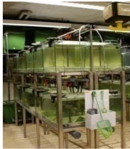
Figure 11: Recirculation system for laboratorial trials
