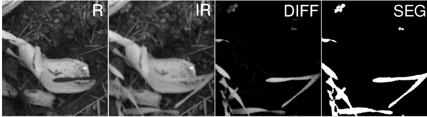
Figure 1.2.: Red (R), infrared (IR) and difference (DIFF) images (histogram stretched for print), (SEG) is the segmented image. The difference images (DIFF) is used for the analysis. Plants appear bright in the infrared and dark in the red image, the background components (soil and crop residues) are dark in the difference image. This can be segmented (SEG) into foreground objects (white) and background.
