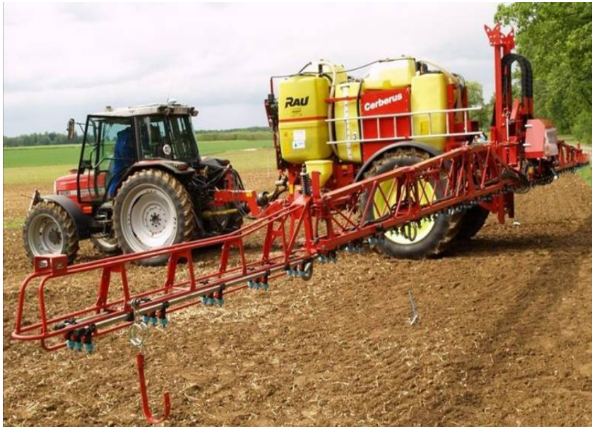
Figure 1.11.: Sprayer with seven boom sections and three separate herbicide tanks (CERBERUS®).
