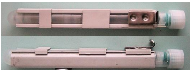
Figure 3.28: The NPC-1 chip dispenser. It was made from a prolonged NPC-1 storage tube and a plastic cable duct. The lid of the cable duct was used to secure the tube and as a movable lid to close the padded dispenser port. The dispenser stored 16 chips. It was refilled by removing the lower cap or by removal of the complete tube.
