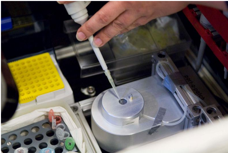
Figure 3.47: Preparation of a patch clamp experiment in the A300 Zero-G (© ESA, Anneke Le Floc'h, 2009)
