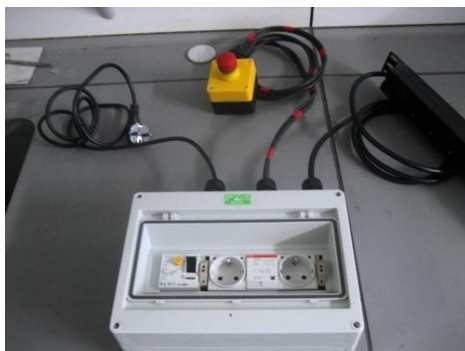
Figure 3.16: The circuitry box with mains plug, emergency stop button and multi-socket.
